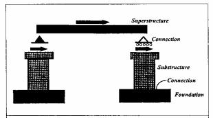
FIG.3 TRANSFER OF FORCES FROM SUPERSTRUCTURE TO SUBSTRUCTURE, AND TO FOUNDATION
