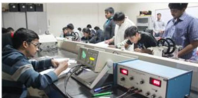
oscilloscopes (Scientech, Scientific and Aplab), signal generators (Scientech, Scientific), dc power supplies and several optical components are available for use
